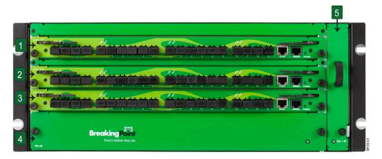
**Callouts 1, 2** and **3** refer to the slots dedicated to high-speed data plane processors (or the blades) for the system. When you initially receive the BreakingPoint 20 chassis, these slots will not contain any blades. You will need to install the blade(s) into the chassis.
