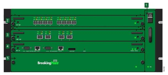
**Callout 1** refers to the removable fan tray that is vertically mounted on the right-side of the chassis.
