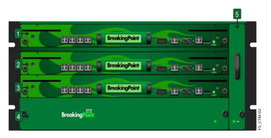
**Callouts 1, 2** and **3** refer to the slots dedicated to high-speed data plane processors (or the blades) for the system. When you initially receive the BreakingPoint FireStorm, these slots will not contain any blades, so you will need to install the blade(s) into the chassis.
