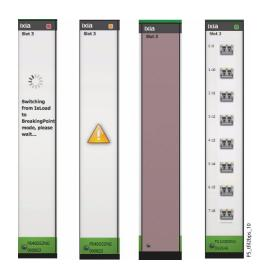
Wait until a green square is displayed in the upper right corner of the load module. Once the green square is displayed, you can begin using the load module or you can begin the transition process for another load module.
